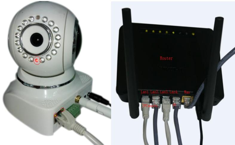
1.3 The software of IP Camera support windows xp/windows8/windows7 etc. operation system, Pls use the power adapter to connect the DC5V port on the back of the ip camera. Plug the other end to an electrical outlet. Check the card's power indicator light (yellow) and the network indicator (green) is working properly, the camera pan and tilt rotate automatically.
